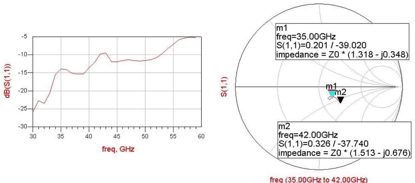
Figure 1: S11 On-Wafer measurements
