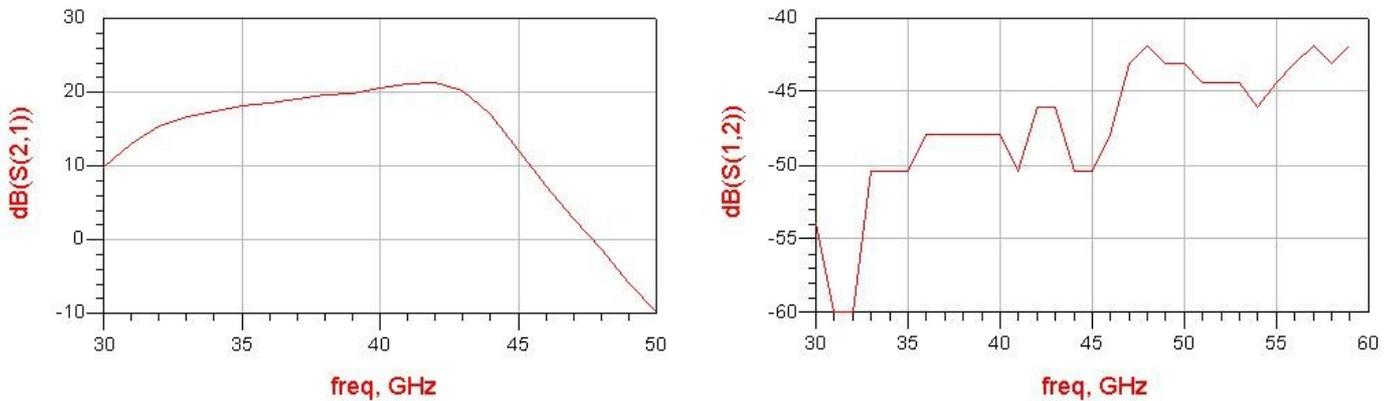
Figure 3: Gain and reverse isolation On-Wafer measurements
