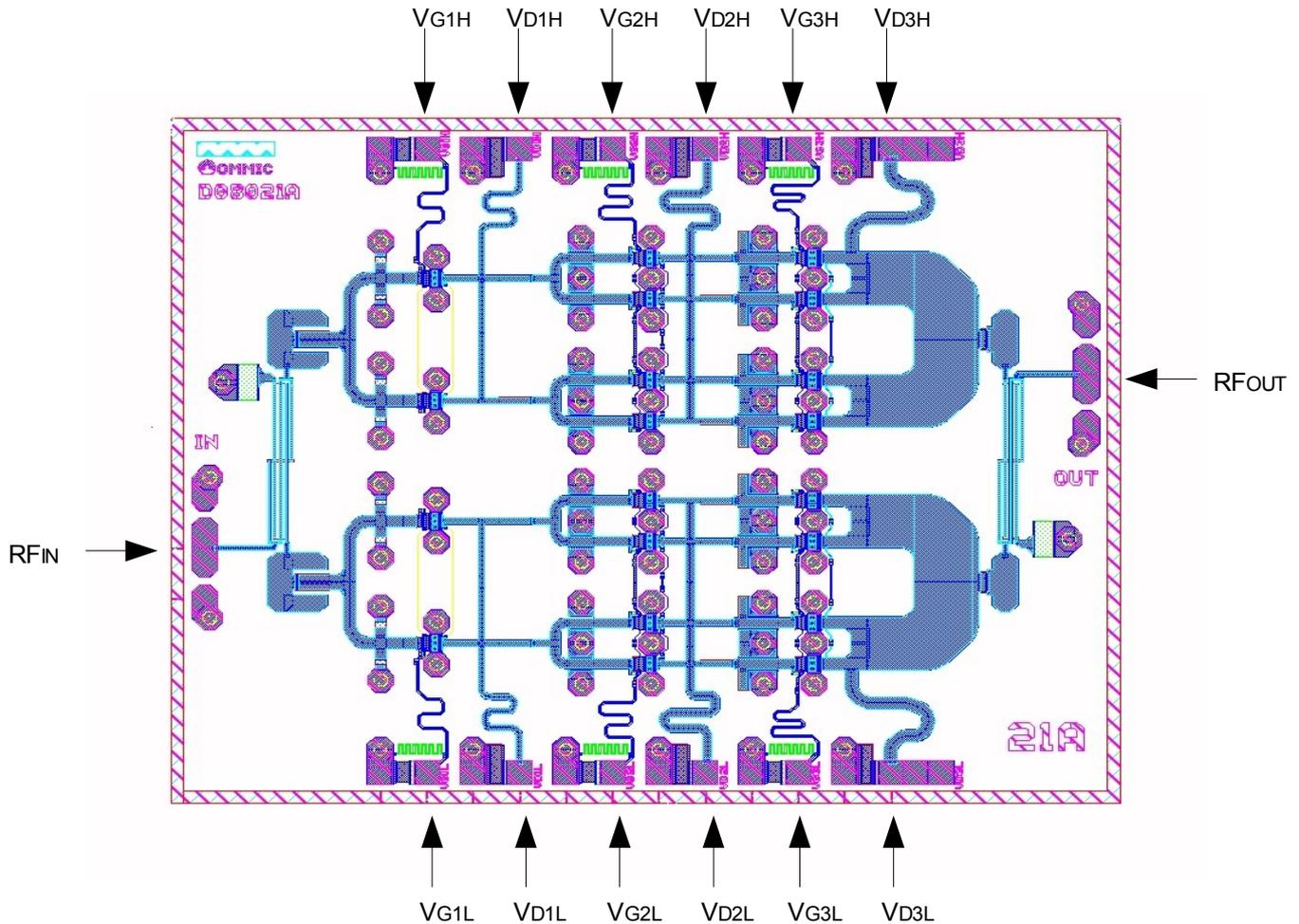
It is highly recommended to place a 47pF RF decoupling chip capacitor C1-C6 and C13-C18 at each DC terminal with as short as possible bonding wires. Additionally for power up, prior to applying drain voltage, gates voltages should be preset to -1,5 V. After applying the drain voltage, transistors should be activated (gate positioned in the -0.3V to 0V range) from the third stage to the first. On shut down, reverse order operation should be performed.
